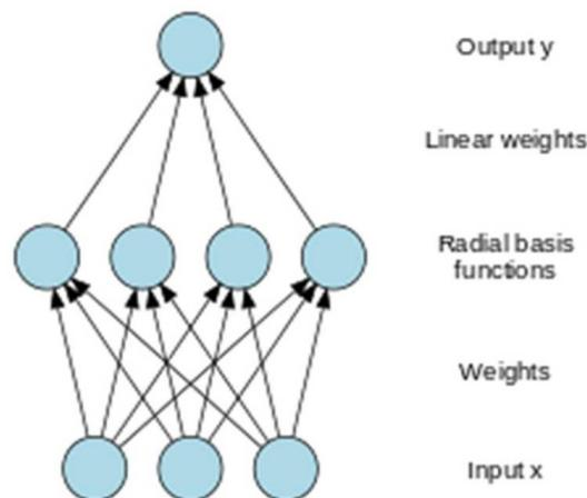
FIG. 8: General Regression Neural Network with Radial Basis Functions.
